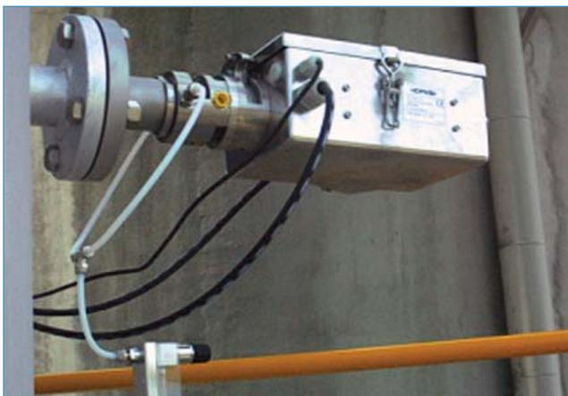
The O2s receiver installed on the stack. The optical fibres transfer the light to the analysers for detection of gaseous compounds.
