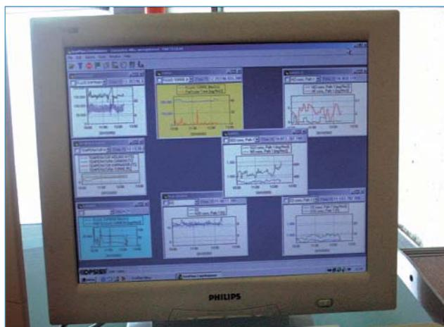
The Oxis EnviMan software handles the data collection, presentation and surveillance from the CEM system. The software is also capable of generating reports.
