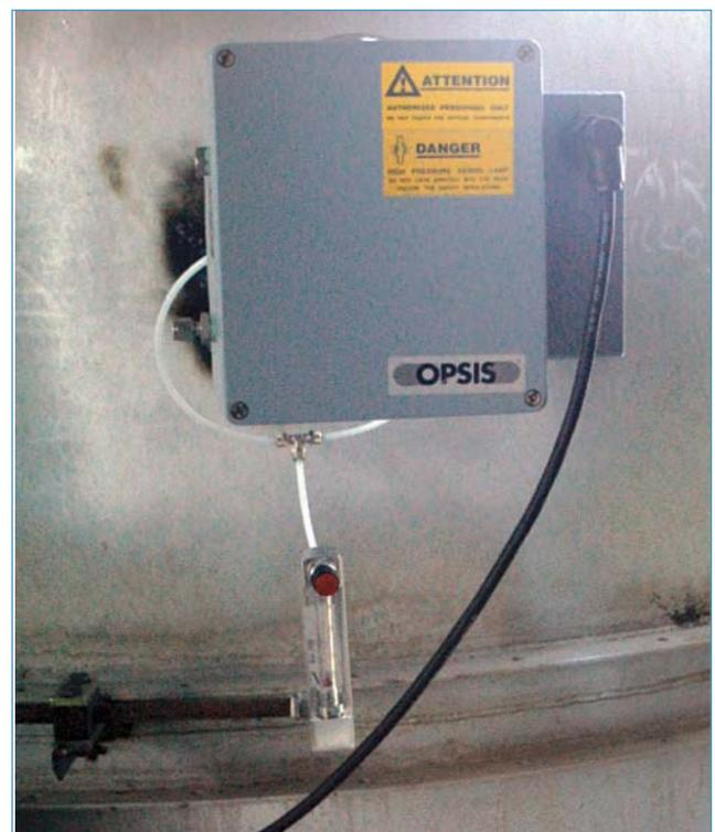
The Opsis emitter including the light source, installed on the stack.
